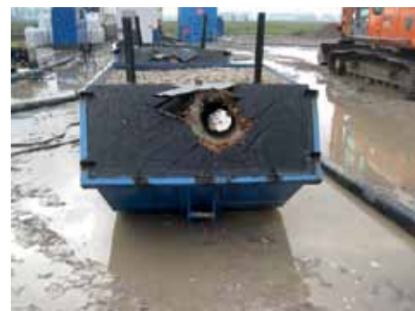
▲ Figure 3: After drilling through biological cemented gravel (left) the borehole remained stable (right).
