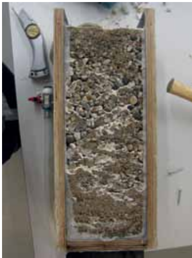
▲ Figure 5 Although the calcium carbonate was heterogeneously distributed throughout the gravel (left), still a clear correlation was observed between the shear strength and the amount of flushes (right).
